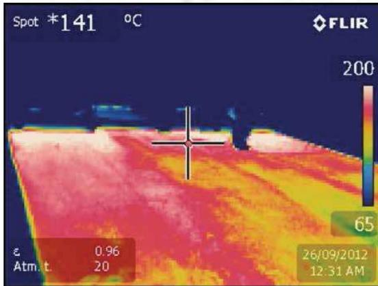
Figure 1 Hot mix asphalt mat temperature of about 141°C
