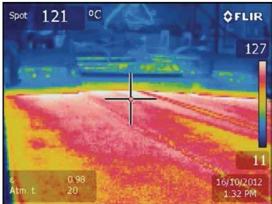
Figure 4 Mat temperatures of warm mix SMA 10
