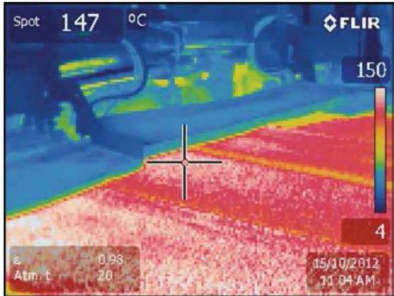
Figure 3 Mat temperatures of hot mix SMA 10
