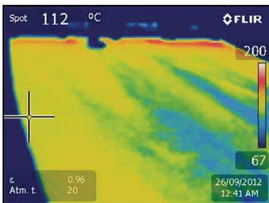
Figure 2 Warm mix asphalt mat temperature of about 112°C
